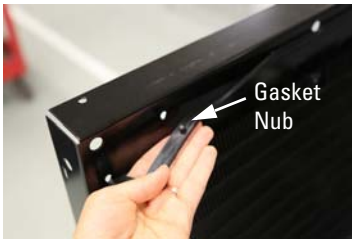
Figure 18: Position gasket on refrigeration module frame and ensure each gasket nub is inserted in corresponding hole
